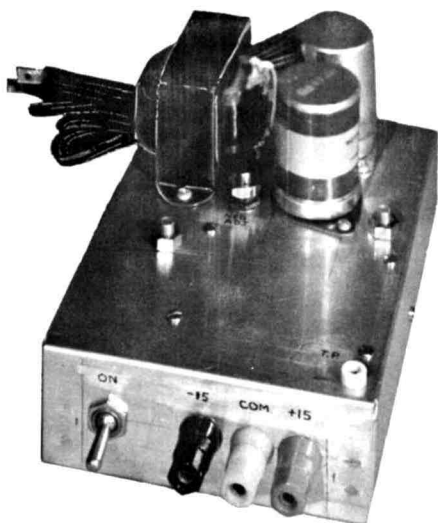
A dual IC-regulated power supply which provides plus and minus fifteen volts.
