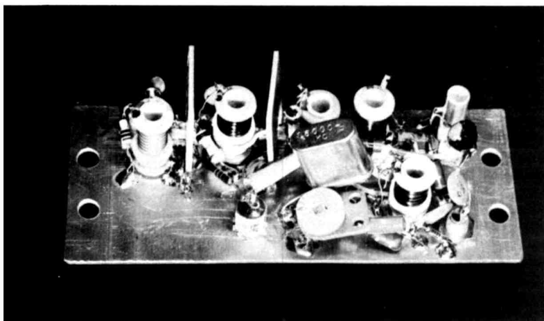
Construction of the FET converter for 50 MHz. Input circuits are to the left.
